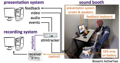
Biosemi ActiveTwo 64 EEG + 4 EOG channels @ 512 Hz
